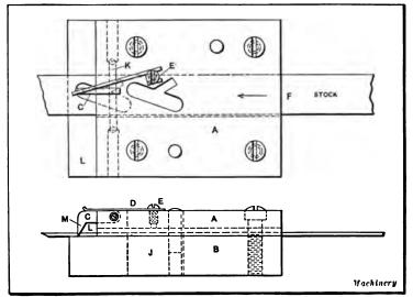
Fig. 35. Latch Stop which is Operated by Feeding Movement of Stock
